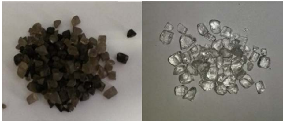
Figure 15. Comparison of recoverable glass fraction after thermal treatment (left) and solvent treatment (right).
