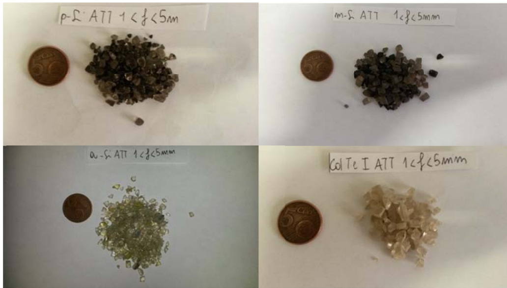
Figure 13. Fractions 1-5 mm for the different panel types obtained after thermal treatment.
