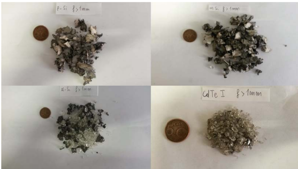
Figure 9. Fractions larger than 1 mm for the different panel types obtained after triple crushing.
