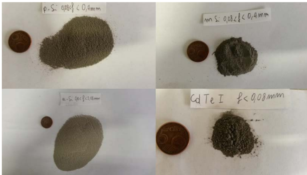
Figure 11. Fractions 0.4-0.08 mm for the different panel types obtained after thermal treatment.
