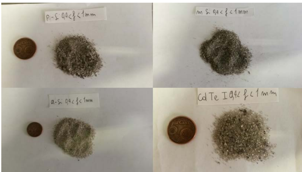
Figure 10. Fractions 0.4-1 mm for the different panel types obtained after triple crushing.
