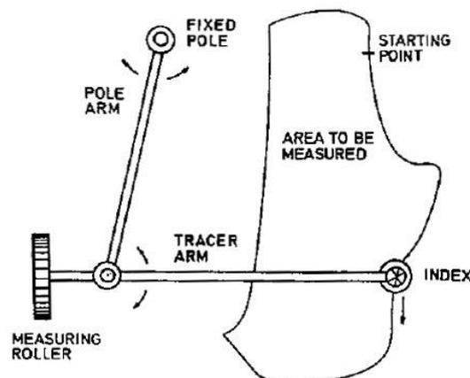
Figure 4 - Main parts of a Polar Planimeter
