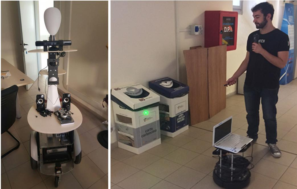
(a) DIAGO, a mobile robot derived from a Segway platform. (b) Turtlebot interacting with human during online semantic mapping.
