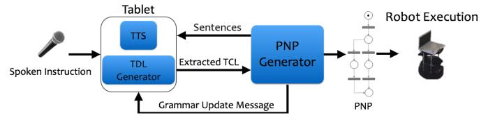
Figure 1: Interaction scheme designed for processing verbal instruction and for generating executable plans.
