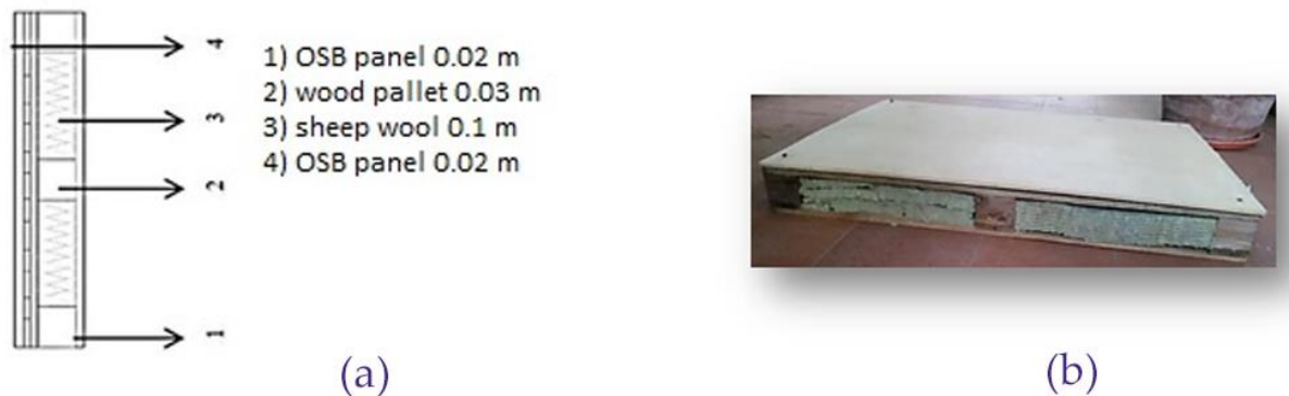
Figure 7. (a) Section of wood pallets model; (b) Wood pallets model prototype.
