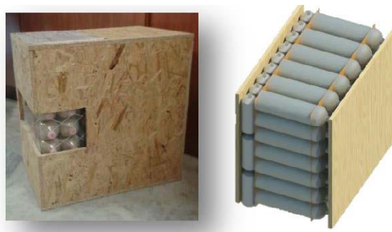
Figure 5. Vertical wall model with plastic bottles prototype and 3D view.
