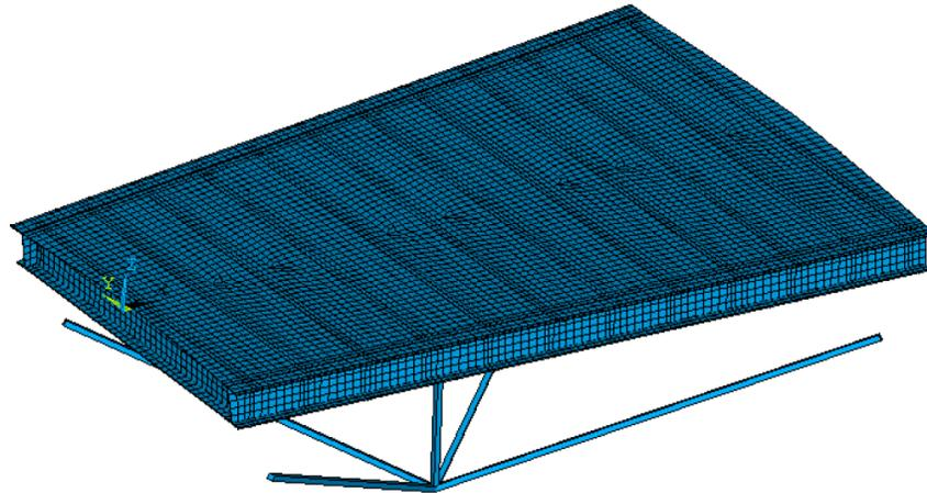
**Figure 3-12: Example of a sub-frame for panels distortion compensation – FEM model**
