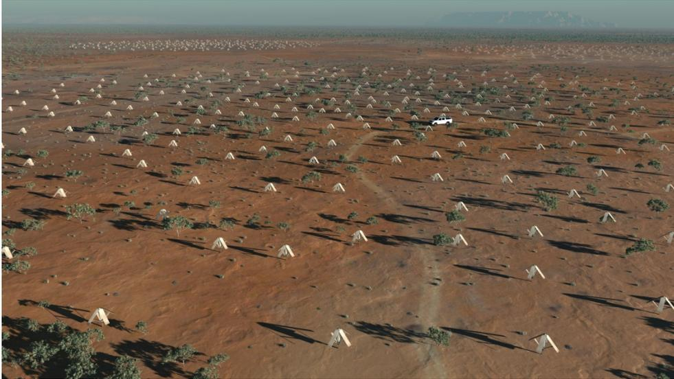
Figure 1-5: A 2D array distribution of antenna elements: the SKA (Square Kilometre Array) – credit to SKA telescope
