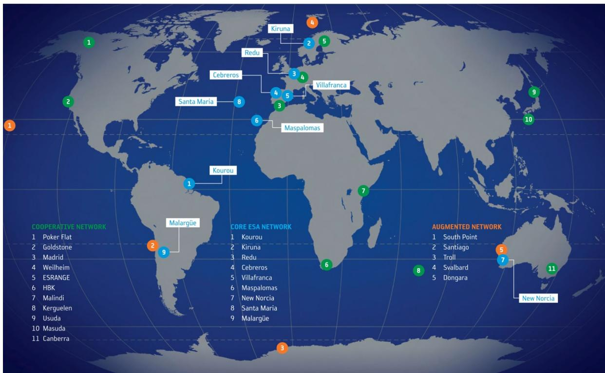
Figure 1-15: ESA ESTRACK core, cooperative and augmented network – credits to ESA
