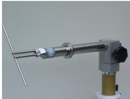
Figure 1-3: A simple dipole antenna – credits to Wikipedia
