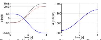
Fig. 1. [Left] Joint position  $q_d$ . Color codes for Figs. 1–3: solid black = joint 1, dashed red = 2, blue with "+" markers = 3. [Right] Joint stiffness  $\sigma_d$  (same profile for all joints).
