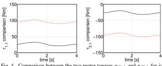
Fig. 4. Comparison between the two motor torques  $\tau_{d1,1}$  and  $\tau_{d2,1}$  for joint 1 with  $\sigma_{d1} = 850$  Nm/rad (solid black lines) and  $\sigma_{d1} = 1275$  Nm/rad (dashed red lines).
