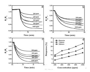
Figure 13: Resistance changes of polyaniline films upon exposure to different vapors in the range 200-1000 ppm: (a): benzene; (b): toluene; (c): xylene (d): linearity of the sensor response with the increase of vapor concentrations. Redrawn and adapted with permission from Ref. [63]
