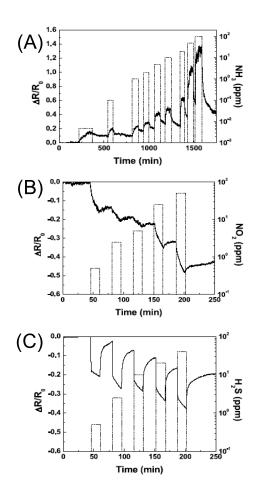
Figure 16: Resistance change  $\Delta R/R_0$  (solid line) and analyte gas concentration (dashed line) as a function of time upon the exposure of different gases. (A): NH<sub>3</sub>; (B): NO<sub>2</sub>; (C): H<sub>2</sub>S. Redrawn and adapted with permission from Ref. [70]
