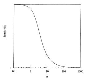
Figure 4: Generalized expression of the gas sensitivity of thin film in terms of the adimenional parameter  $m=L\sqrt{\frac{K_m}{D}}$ . Reproduced with permission from Ref. [44]
