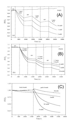
Figure 14: Real time impedance  $Z/Z_0$  response of PANI/AuNPs sensors prepared with 1, 5, 10 mM HAuCl<sub>4</sub>concentration upon exposure to H<sub>2</sub>S (1 ppm) (A) and CH<sub>3</sub>SH (1.5 ppm) (B). Typical impedance response of sensors at different HAuCl<sub>4</sub> concentration to the expired breath of a healthy volunteer after ingestion of raw garlic. Redrawn and adapted with permission from Ref. [68]
