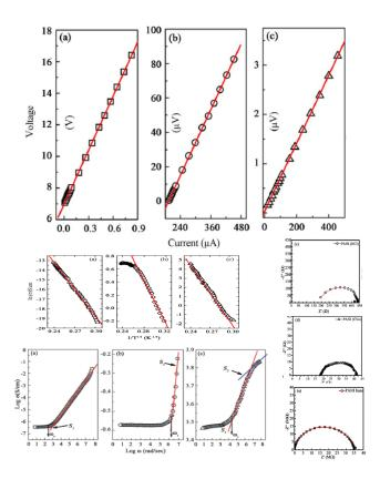
Figure 3: Upper panels: Current-Voltage characteristics of (a) PANI base, (b) PANI (HCl) and (c) PANI (CSA). Intermediate panels: Arrhenius plots for (a) PANI base, (b) PANI (HCl) and (c) PANI (CSA). Bottom panels: Frequency dependent electrical conductivity  $\sigma(\omega)$  for (a) PANI base, (b) HCl and (c) CSA doped PANI.  $\omega_c$  indicates the DC-AC transition. On the right, Nyquist plot of (a) PANI base, (b) PANI (HCl) and (c) PANI (CSA). Reproduced with permission from Ref. [39]
