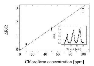
Figure 12: The maximum of the response of Cu-PANI to exposure of chloroform at various concentrations (from 0 to 100 ppm). The inset shoes the temporal response Sensor was exposed to chloroform vapors for 5 min and to dry air for 5 min, alternately. Redrawn and adapted with permission from Ref. [62]
