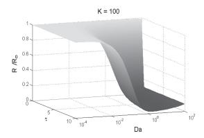
Figure 6: Results of the reaction-diffusion model showing the ratio  $R/R_0$  of the resistance prior and after the exposure plotted as a function of the Damköhler constant  $D_a$  and the dimensionless time  $\tau$  for a selected value of the equilibrium constant  $K = k_f/k_r$  (K=100). Reproduced with permission from Ref. [51]
