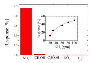
Figure 10: Response of PANI-TiO<sub>2</sub> sensor film to NH<sub>3</sub> (concentration 20 ppm), CH<sub>3</sub>OH (concentration 100 ppm),  $C_2H_5OH$  (concentration 100 ppm), NO<sub>2</sub> (concentration 100 ppm), H<sub>2</sub>S (concentration 100 ppm). The inset shows the response of the sensor to NH<sub>3</sub> as a function of concentration in the range 20-100 ppm. Redrawn and adapted with permission from Ref. [57]
