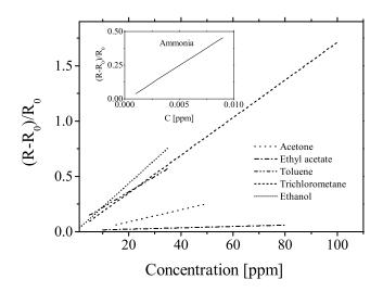
Figure 17: Response to various volatile organic compounds for PANI coating onto porous non-woven fabrics. Redrawn and adapted with permission from Ref. [76]
