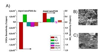
Figure 15: A): Sensitivity of nanoPANI-Au and nanoPANI for ammonia, ethanol, toluene and acetonitrile. B): SEM image of nanoPANI-Au composite obtained from osmosis-based method. (nanoparticles with diameters in the range from 180 to 220 nm). C): SEM image of nanoPANI. Redrawn and adapted with permission from Ref. [69]
