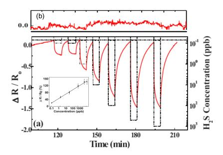
Figure 7: (a): Transient response  $\Delta R/R_0$  of gold nanoparticle functionalized PANI nanowire network based chemiresistive sensors towards 0.1, 1, 10, 100, 500 and 1 ppb concentration of H<sub>2</sub>S gas. The inset shows the response  $\Delta R/R_0$  as a function of H<sub>2</sub>S concentration. (b): response of unfunctionalized PANI nanowire network towards 50 ppb of H<sub>2</sub>S gas. Reproduced with permission from Ref. [52]
