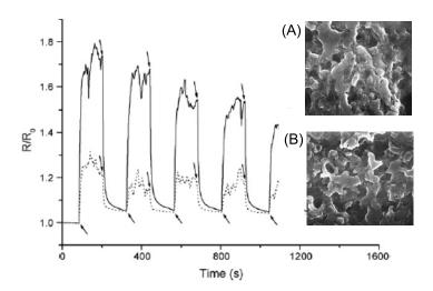
Figure 9: The effect of ethanol vapor on the resistance of P film (full line) and F film (dotted line). Redrawn and adapted with permission from Ref. [53]
