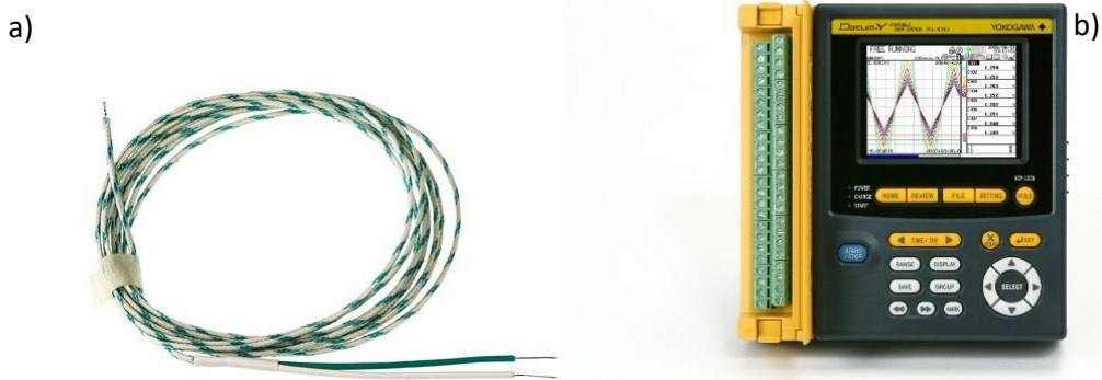
Figure 47 Thermocouple and datalogger
