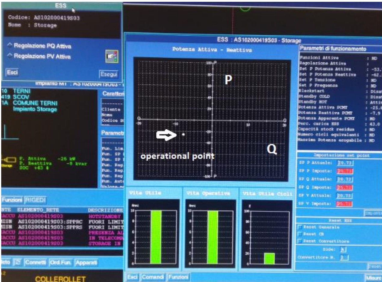
Figure 111. SCADA HMI interface during a (P,Q) request
