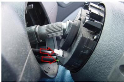
Figure 7: Steering angle sensor.
