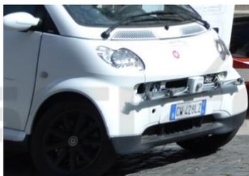
Figure 3: Radar and ultrasonic sensors installed on the front of the vehicle.
