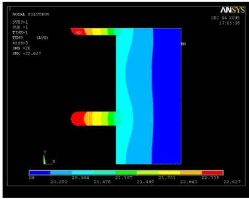
Figure 6: Thermal field in the  $\pi$ -mode cavity.
