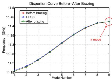
Figure 4: Dispersion curve before and after brazing.
