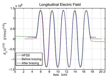
Figure 5: Measured longitudinal electric field on axis.
