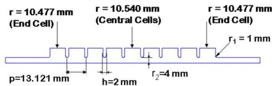
Figure 1: 2D profile of the X-band structure.
