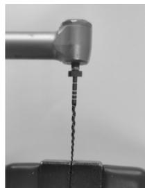
**Figure 2.** Device for torsional resistance tests.
