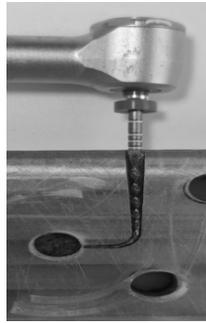
**Figure 1.** Device for cyclic fatigue resistance tests.
