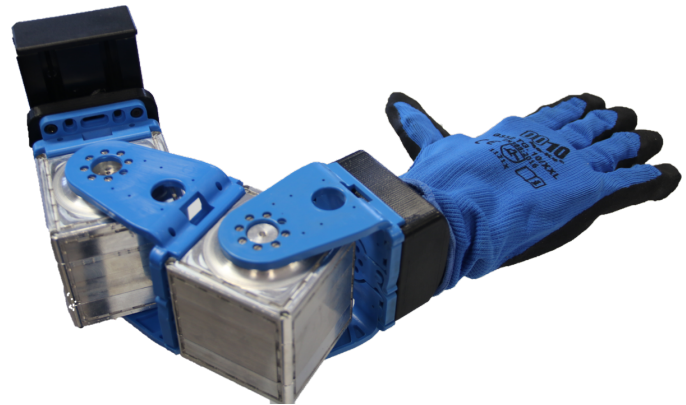
Fig. 1. Planar 2R manipulator, powered by two series elastic actuators and equipped with a soft end-effector.
