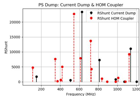
Figure 6: Shunt impedances calculated from the Eigenmode solutions of the PS dump model with the tapers and coupling loops compared to the presently installed PS dump.
