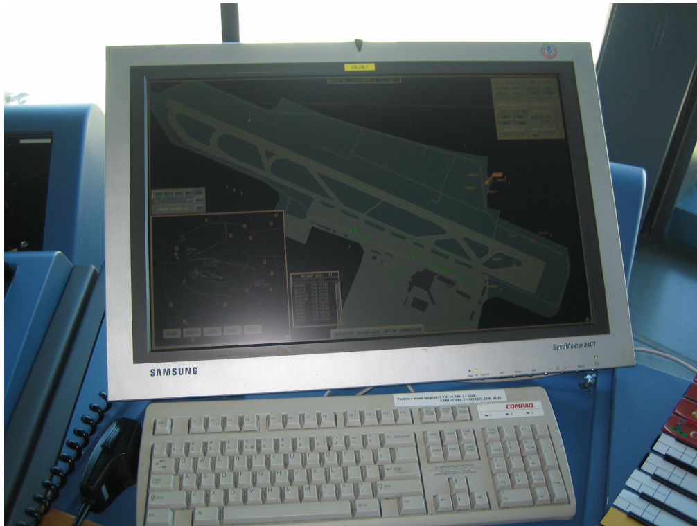
Figure 6 – What the approach controller sees, from the A-SMGCS console in tower
