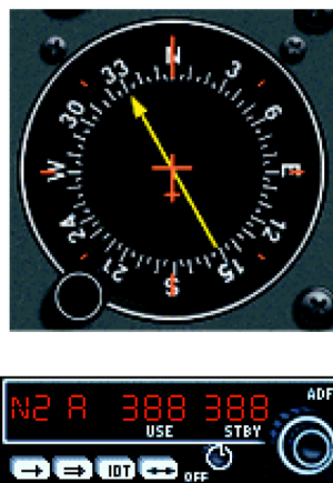
Figure 9 – ADF indicator instrument and receiver [ATC-4]
