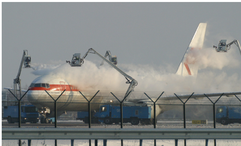
Figure 7 – De-icing operations increase the time required between flights and reduce airport capacity
