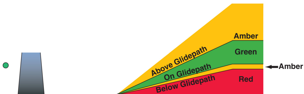
Figure 6 – Tri-color visual approach slope indicator [ATC-3]
