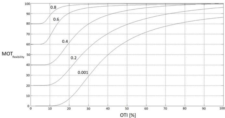
Figure 6:  $MOT_{flexibility}$  as a function of the percentage of OTs that can be integrated into the IoE system (OTI), for different values of initial  $MOT_{flexibility}$  (0.001, 0.2, 0.4, 0.6, 0.8).
