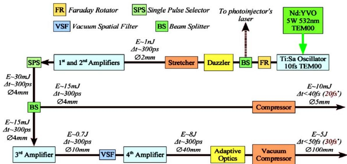
Figure 1: Lay-out of the FLAME Laser System.
