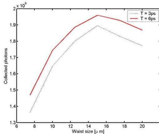
Figure 6: X-ray yield vs. laser spot size and pulse length
