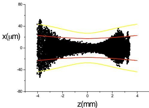
Figure 4: Electron bunch and laser pulse overlap at the final focus in the collision point
