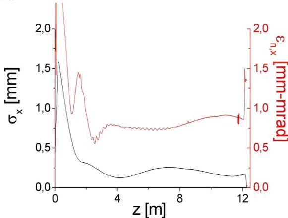
Figure 3: Beam emittance and envelope along z
