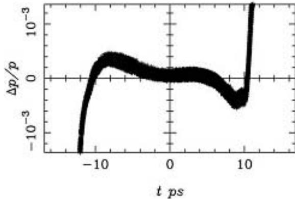
Figure 2: Longitudinal phase space distribution at Linac exit.
