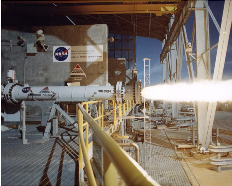
Figure 3: Amroc HRE firing test at NASA Stennis Space Center in 1994 (Credits NASA).
