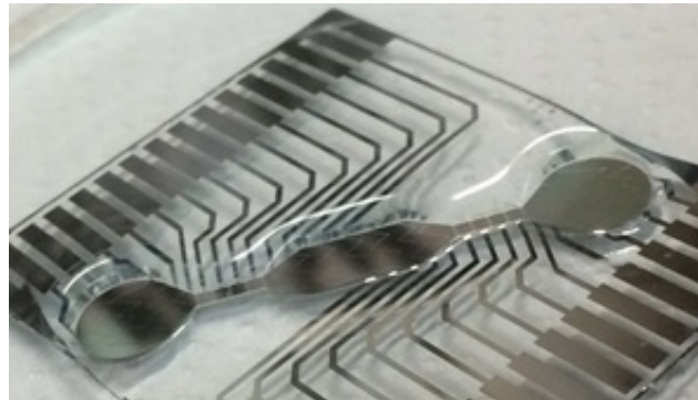
Figure 1.6. Bottom glass: water covers the glass except for the electrodes that are covered by the hydrophobic layer.
