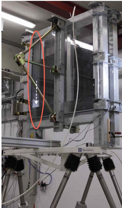
**Figure 2.1.** View of the sloshing tank. The red ellipse highlights the stainless steel wall holding the deformable plate, indicated by the white arrow.
