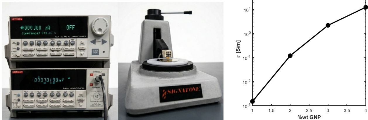
Fig. 2.3 Four-point probe DC resistivity measurement setup (left) and resulting electrical percolation curve (right) as a function of GNP content in the AZ paint.
