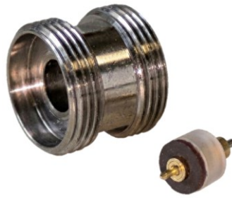
Fig. 4.3 Coaxial airline with thin film loaded on rigid substrates inserted on the central pin of the coaxial airline.
