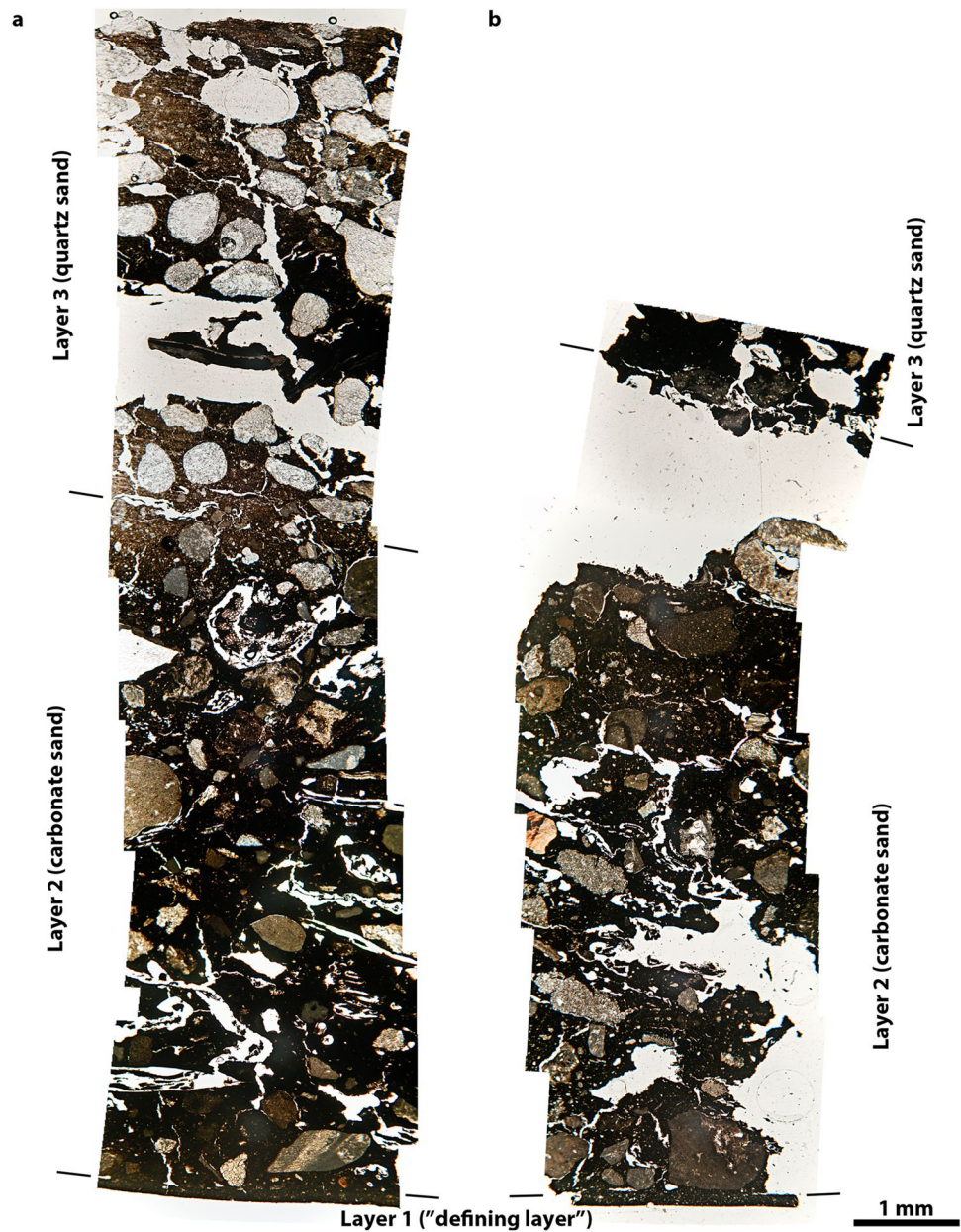
Fig. 10 Cross-sections through (a) the complete mould of experiment 3 (Exp3-M3); (b) the mould of experiment 4 with the outer layer detached during sampling and the outer part of this layer missing (Exp4-M3). The approximate locations of the interfaces between the layers are indicated, composite images
