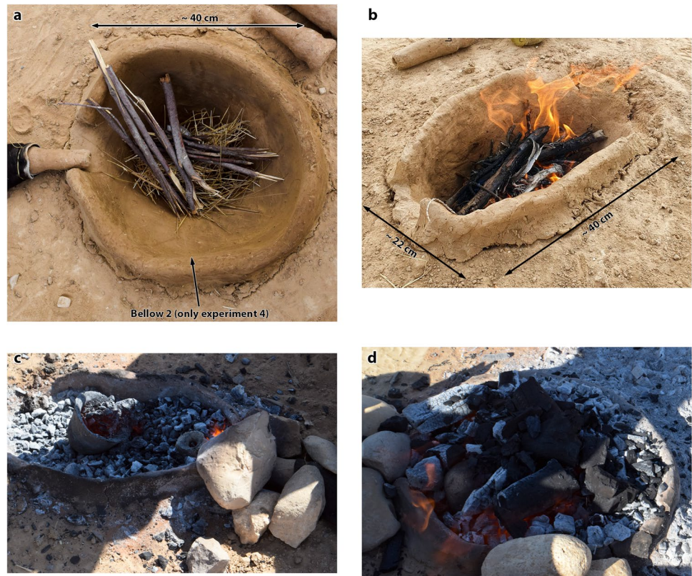
Fig. 4 The furnaces used in the experiment to fire the moulds: (a) the furnace to melt the metal in a crucible before kindling the fire; the later position of bellow 2 is indicated. (b) The furnace for de-waxing. (c) The location of the moulds from experiments 1 to 3 in the furnace for wax removal. (d) The crucible furnace with the mould from experiment 4 placed between the tuyères. The tuyères are located under the cobblestones
