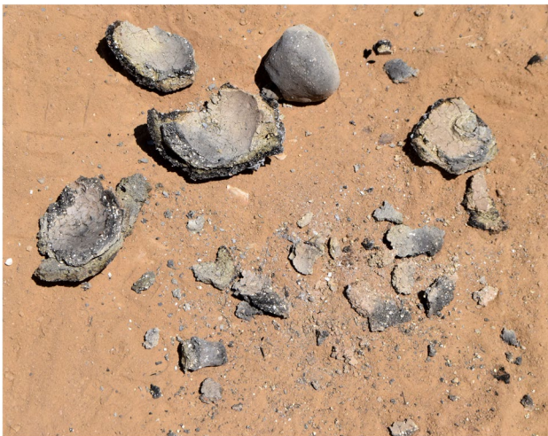
Fig. 6 The mould of experiment 1 after it was accidentally broken in the field. The separation of layers 2 and 3 is apparent in the larger fragments
