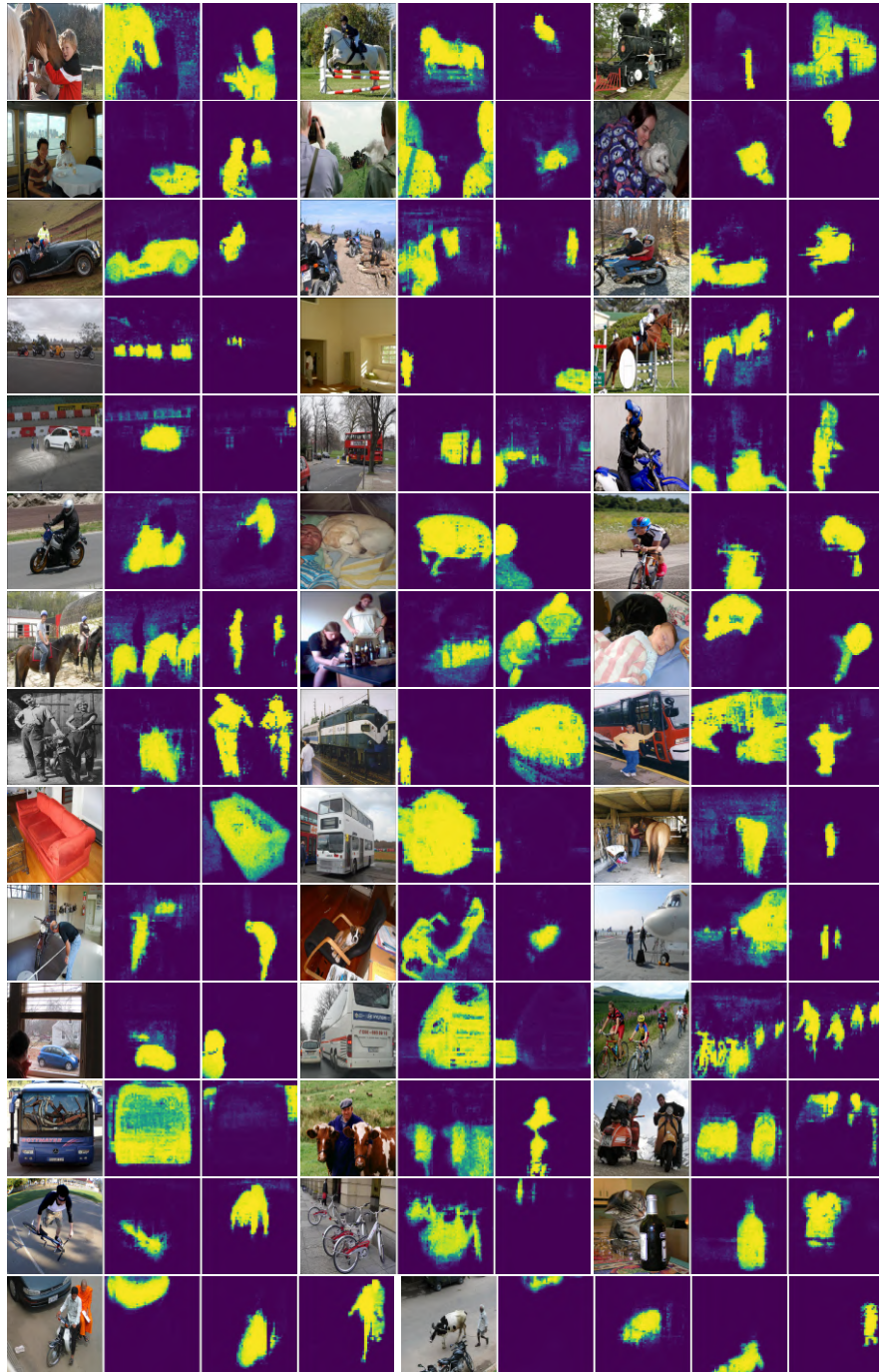
Fig. S1: Each row shows the original images (two or three per row) and the BPM for each class appearing in the image on its right. The BPM of size 60 \times 60 are resized to the original image size.
