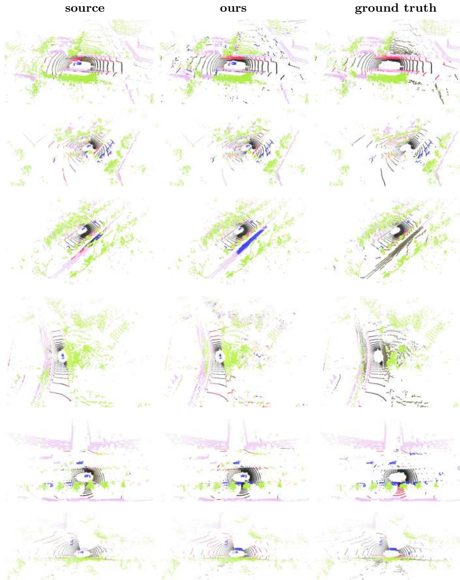
Fig. 5. Qualitative adaptation results on Synth4D \rightarrow nuScenes reporting large improvement cases. We compare GIPSO predictions during SF-OUA (ours) with source model predictions (source) and with ground truth annotations (ground truth).
