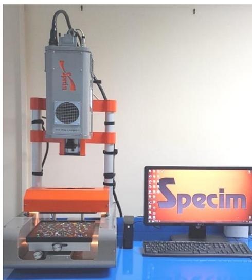
Figura 4.1. Sisuchema XLTM workstation (Specim Ltd.).
