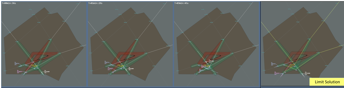
Figure 4: Storyboard presentation of the proposed solution. The sequence of images 1 to 3 shows the temporal steps to solve the conflict. The limit solution shows the good solution but with is close the minimum separation criteria between conflicting aircraft.
