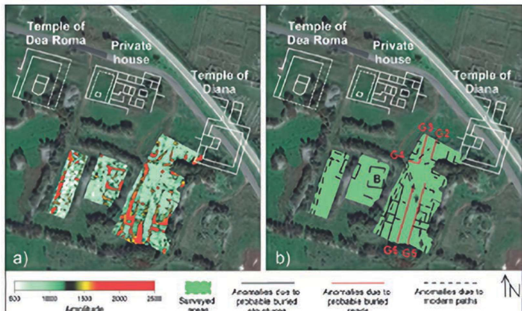
Fig. 2. GPR results in the southern part of the private houses: time slice relative to the time window 14-18 ns (about 0,7-1,4 m in depth), overlapped on the photogrammetric image (a) and identification of anomalies (b) [Cuzzolino, Gentile 2019].
