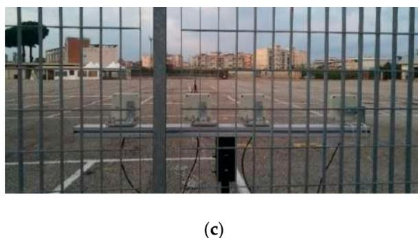
Figure 21. Acquisition geometry: (a) sketch of the transmitter and receiver configurations (b) Wi-Fi access point transmitter to be located, and (c) receiving array geometry with  $N = 4$  Wi-Fi antennas.
