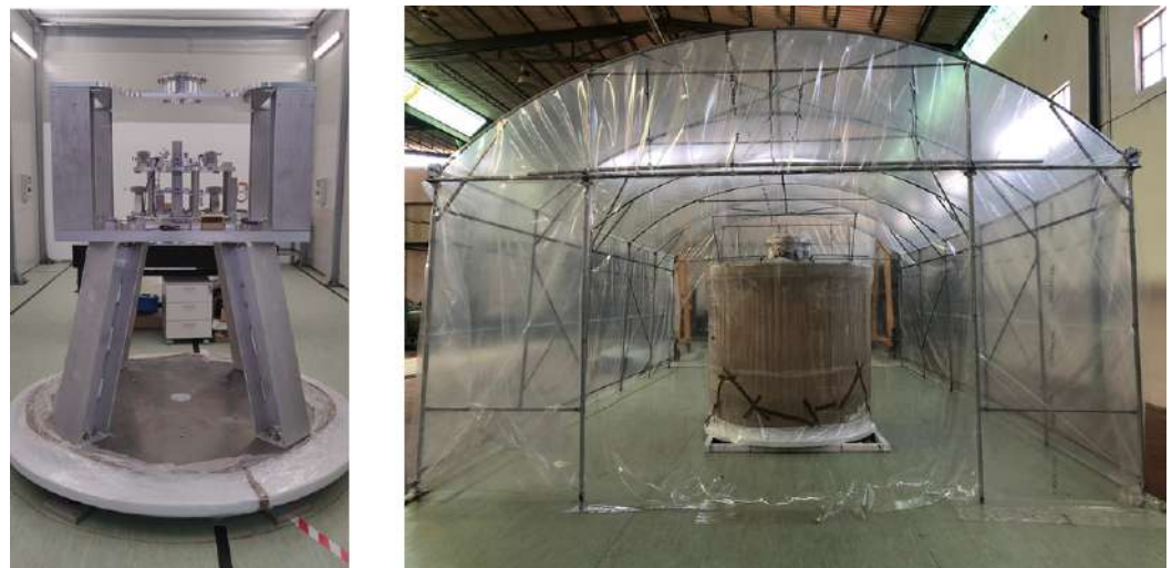
Figure 17. (Left): Picture of the final setup (still under construction) positioned on a solid table grounded to the cryostat basis. It is positioned inside the Archimedes hangar. (Right): Tent structure hosting the cryostat cover.
