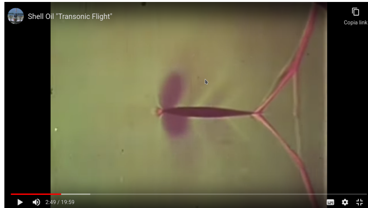
Figure 9.1. Transonic fish-tail: experimental visualization re-printed from [208].
