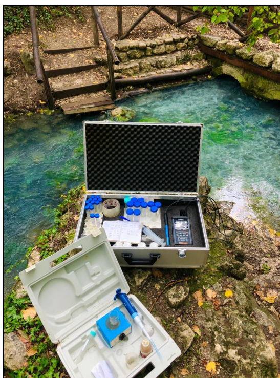
Figure 3.3. Material for survey sampling (i.e., polyethylene bottles for collecting water, and the multiparametric probe WTW Multi 3420 right inside the case) and in situ determination of alkalinity.
