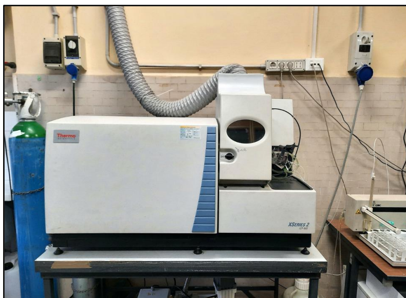
Figure 3.5. Spectrometer ICP-MS (Inductively Coupled Plasma Mass Spectrometry) used for trace element analyses.
