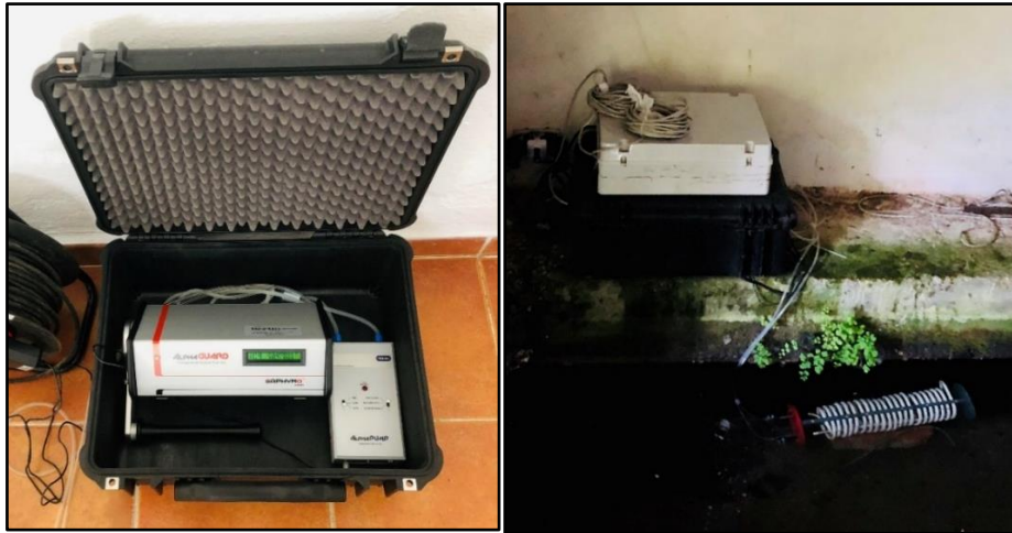
Figure 3.6. The AlphaGUARD device (Model PQ2000PRO) for radon monitoring with a RAM 7 module for stripping gas from the water.
