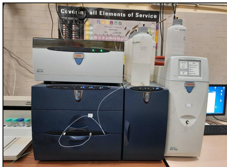
Figure 3.4. The Chromatograph Dionex ICS 1100 for cations analyses and the Chromatograph Dionex ICS 5000 for the anions analyses, equipped with a Dionex AS-DV autosampler.
