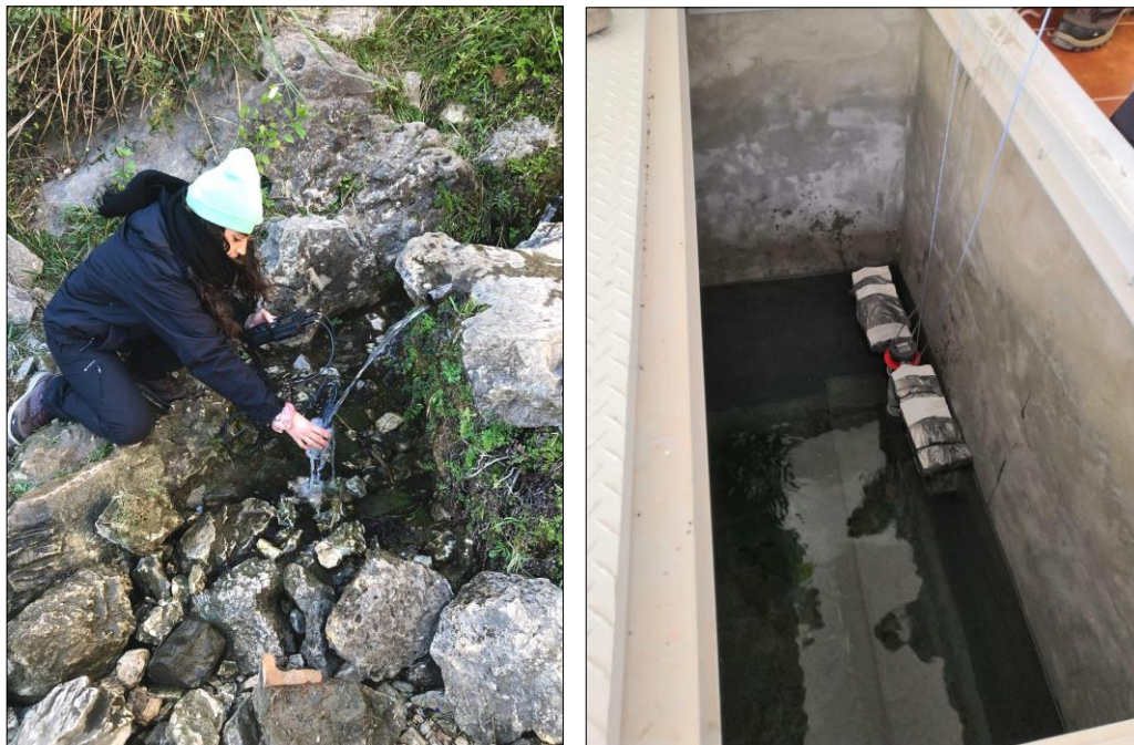
Figure 4.17. On the left, me sampling groundwater; on the right, the AlphaGUARD device for radon monitoring that I installed at Maro spring.
