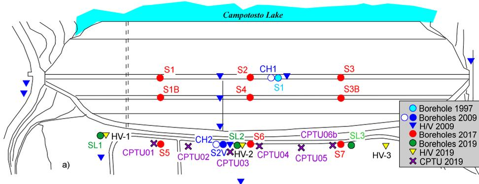
Figure 8 Plan view of Poggio Cancelli dam showing exploration locations.
