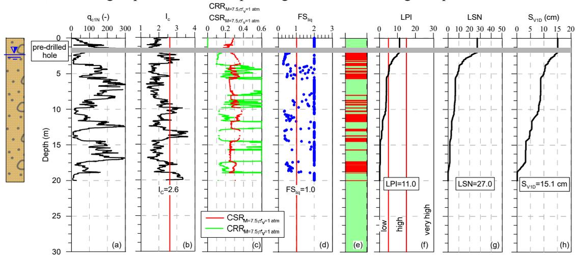
Figure 13. Results of the Idriss and Boulanger (2015) liquefaction procedure for estimation of safety factor against liquefaction ( $FS_{liq}$ ) and integral parameters LPI, LSN and  $S_{VID}$  (red bars indicate zones with  $FS_{liq}<1$ )
