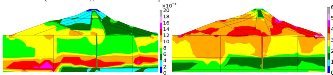
Figure 12. Contours of shear strain (left) and damping (right) - average of 7 earthquakes.
