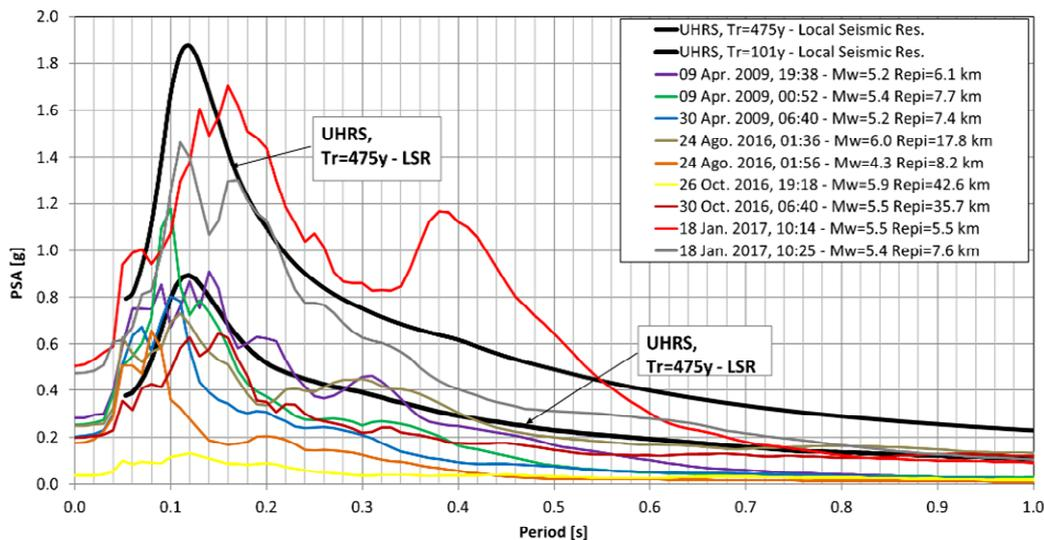
Figure 9: Response spectra of the accelerometric components (average between EW and NS directions) recorded at the PCB station and reference spectra calculated with LSR analysis (solid black line).
