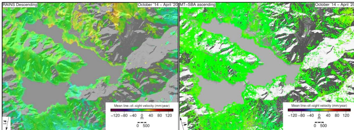
Figure 7. Results of the areal InSAR analysis for the entire analysis period (October 2014 to April 2020). The interferometric stack on the left shows the results of the standard two-pass interferometric analysis (RAINS) obtained for the descending geometry. The results of the multi-temporal analysis (MT-SBA) are shown on the right by means of stable reflectors obtained for the ascending geometry.
