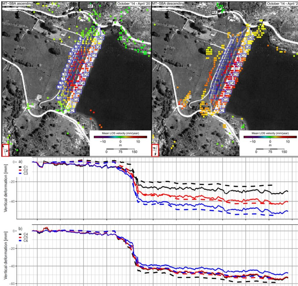
Figure 10. Results of the site-specific InSAR analysis of the Poggio Cancelli dam. The upper aerial photograph reports the pixels corresponding to stable reflectors and their average displacement rates during the analysis period. The graphs report the cumulative vertical displacements (ground measurements vs. InSAR)
