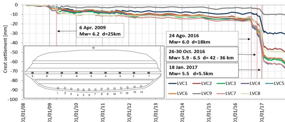
Figure 6. Displacements trends of the Poggio Cancelli embankment crest before and after the seismic sequences 2009 and 2016-2017.
