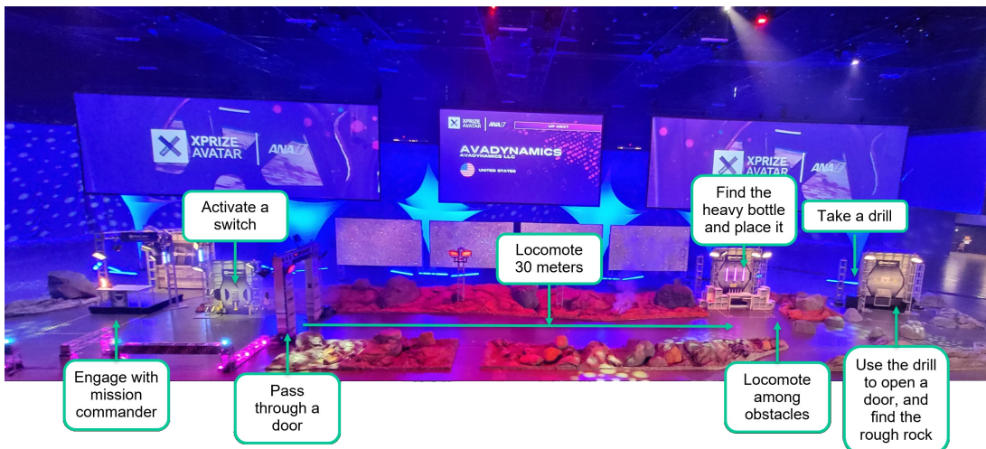
Figure S2: A representation of the ANA Avatar XPrize finals course. It is themed on the exploration of another planet. The labels indicate how the tasks listed in Table 2 were executed on the course.
