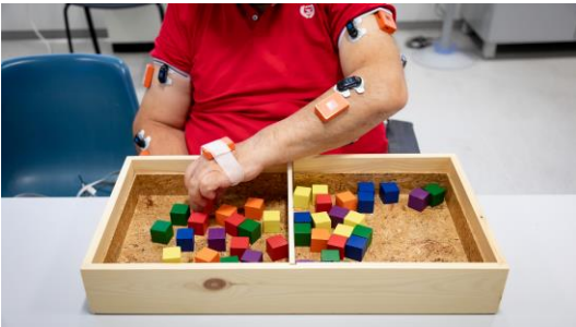
Fig. 1 – Experimental setup: Box and Block Test kit (rectangular box and cubes), 16 wireless sensors (in black) and 8 IMUs (in orange) for collecting EMG and kinematics data, respectively.
