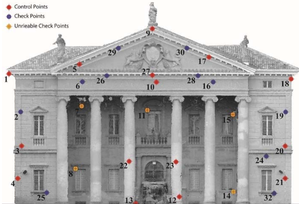
Figure 5. GCPs network distributed on the façade.
