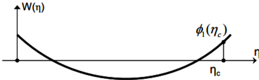
FIG. 9 – Mode shape for the case of a “free-free” beam See [4]
