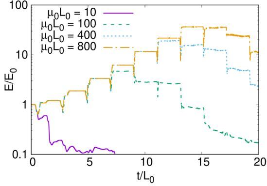
FIG. 2. Evolution of the integrated energy of a scalar inside an oscillating star, for different bare mass parameters  $\mu_0$ . The coupling to matter is such that the field is massless inside the star ( $\mu_{\text{in}} = 0$ ). The field sees only an oscillating boundary with  $\omega L_0 = 3.1$ ; we froze density variations inside the star. The initial data is characterized by  $\sigma = 0.1L_0$ .
