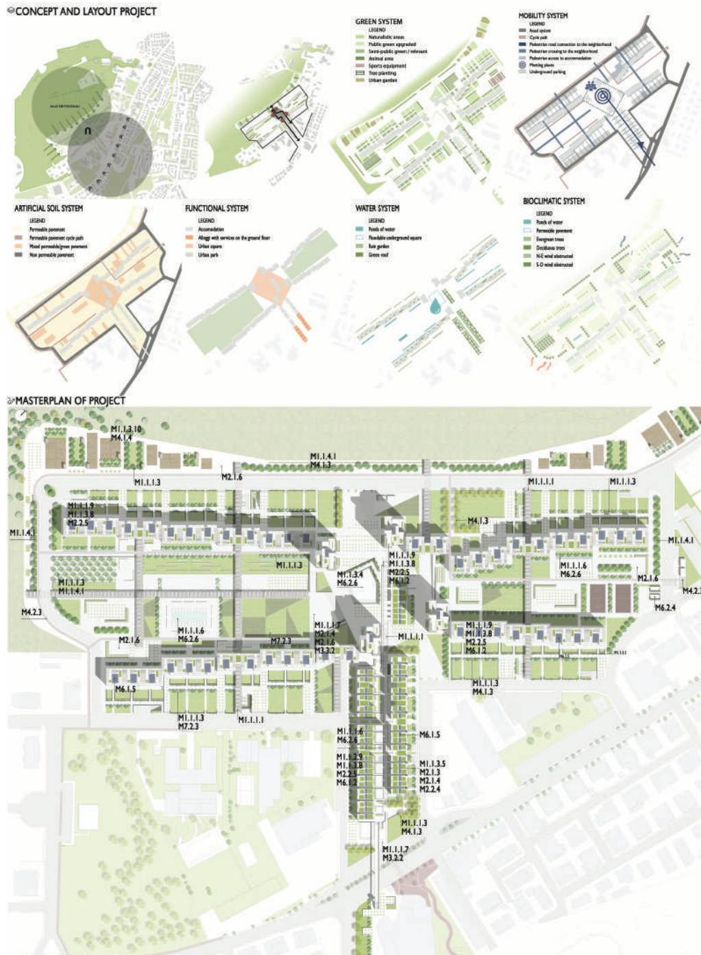
Fig. 8 – Masterplan of the former IACP neighbourhood of Torrevecchia, indicating the Strategies and intervention Measures, and specific Actions of retrofitting of the public spaces subject to modelling and simulation
