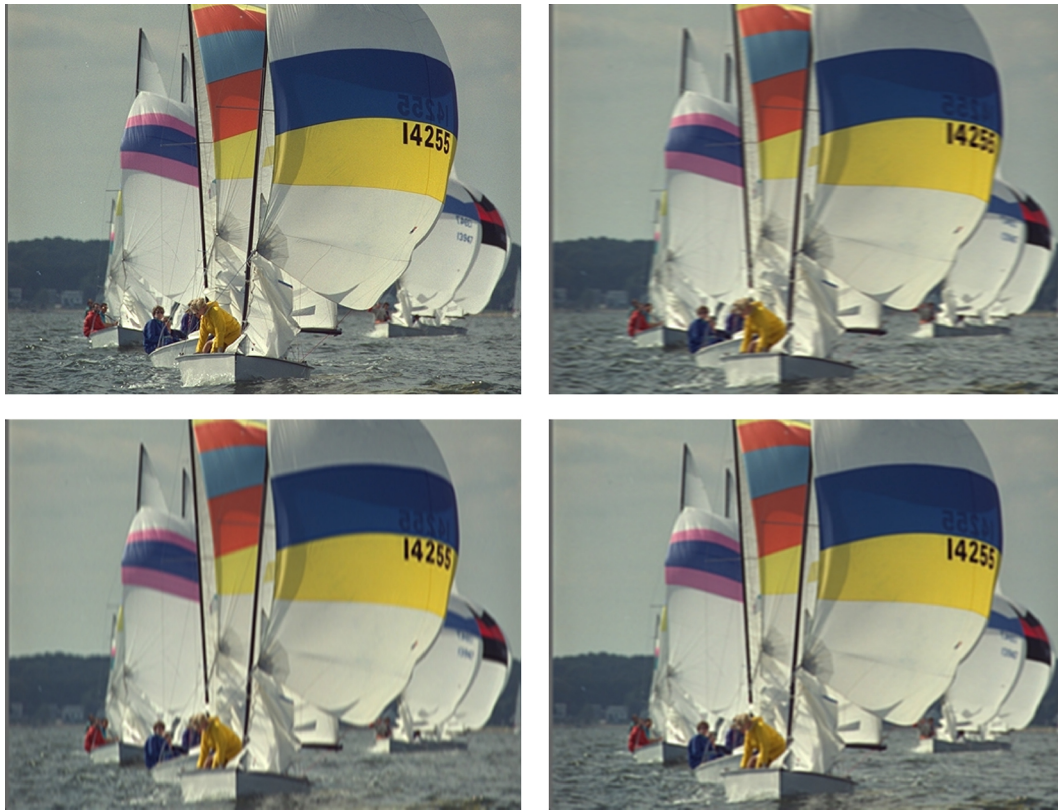
Fig. 6. A unblurred image (upper left) and its astigmatic blurred versions. For s_H = 4, s_V = 1 (horizontal blur, upper right), and for s_H = 1, s_V = 4 (vertical blur, lower left). They are PFI equivalent to the isotropic Gaussian blurred version shown in the lower right image with s_B = 2.54 .
