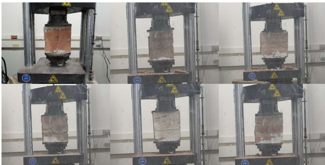
543 544 545 Figure 21 – URM prisms extracted from the Dillon Hall.
