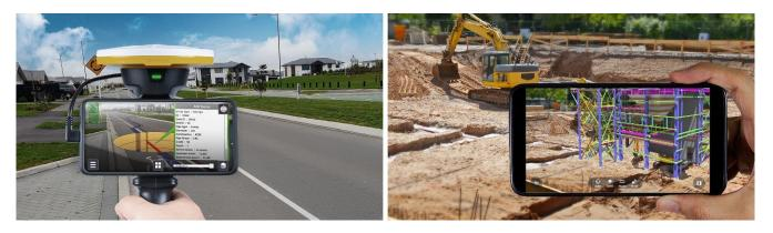
Figure 5. Trimble SiteVision AR system (left) and smartphone-based AR (right).
