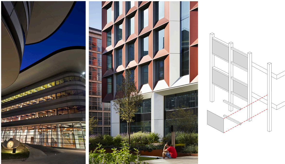
Figure 2.7: Assembly diagram and application examples of a stick curtain wall system
