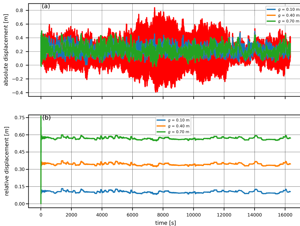
Figure 7.42: Top floor absolute displacement of MF-equipped building (a) and top floor relative displacement of multiblock MF (b) for variable initial gap, g
