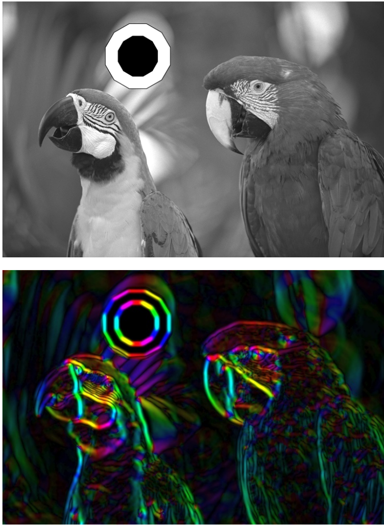
Figure 6.3. The luminance of an image (left) of the database LIVE [81] compared to the corresponding visual map y(\mathbf{p}) (right), where the magnitude of the edges is coded into luminance, and their direction, in the interval [0, \pi) , into hue. The hue/direction code is read in the edges of the upper-left superimposed polygonal.
