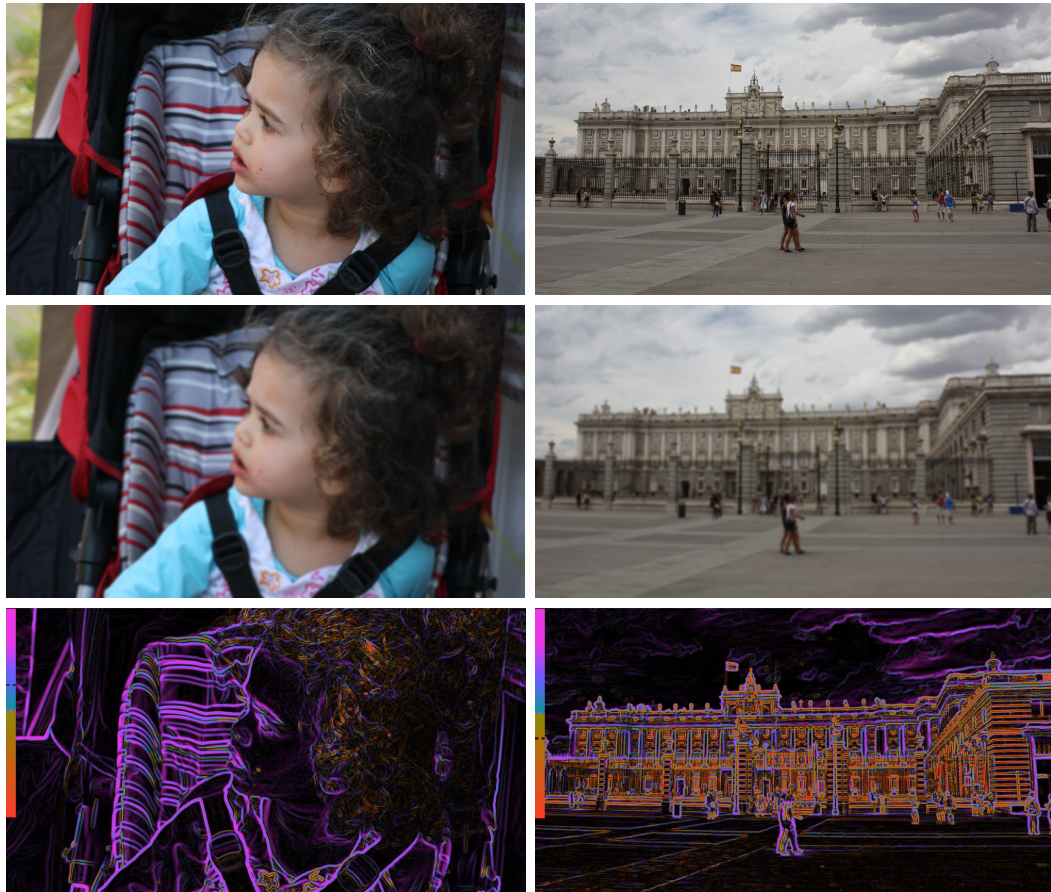
Figure 10.5. Upper row: two original images. Second rows: Gaussian blurred images. Lower rows: certainty maps. The images in the left column correspond to an image judged with very low DMOS (high quality), on the other hand, in the right column with very high DMOS (low quality). It is possible to appreciate a high dominance of purple which represents greater certainty, in the image with higher quality (left column), and a high dominance of reds which represents greater loss, in the image with worse quality (right column). The isoluminance colors maintain a constant intensity at the same edge level, so, only the weight defines the local contrast. The blur levels are s_B = 2.4 for the left column image and s_B = 2.5 for the right column image.
