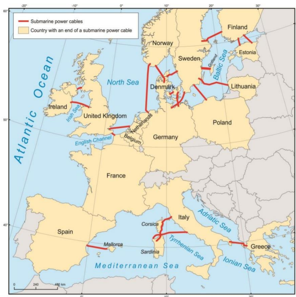
Figure 4.1 Submarine power cables in Europe [ adapted from 53]
