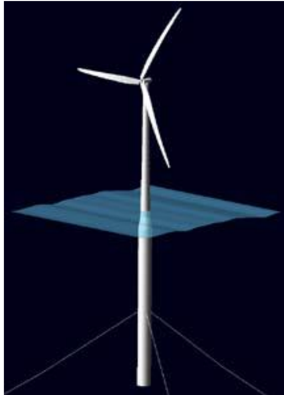
Figure 5.2 OC3 Hywind FOWT [adapted from 49]
