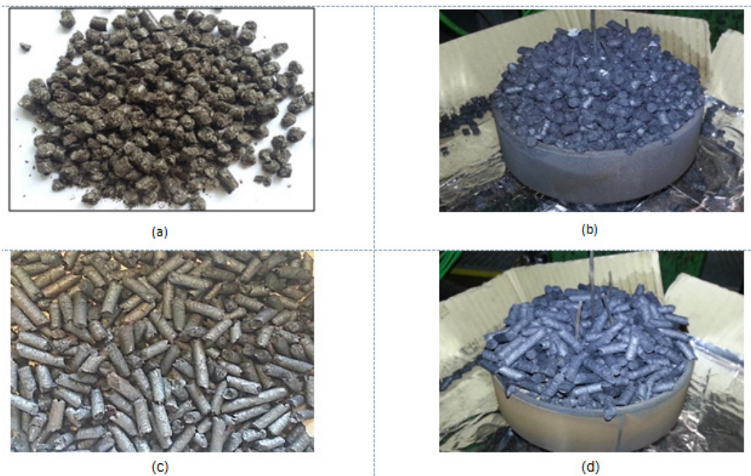
Fig. 4. Pictures of feedstock investigated in the batch reactor: GV sample before (a) and after (b) and SFH before (c) and after (d) the test runs.
