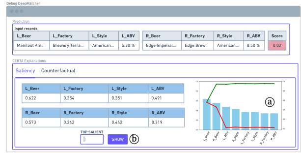
Figure 3: Debugging a DeepMatcher's prediction with saliency explanations.
