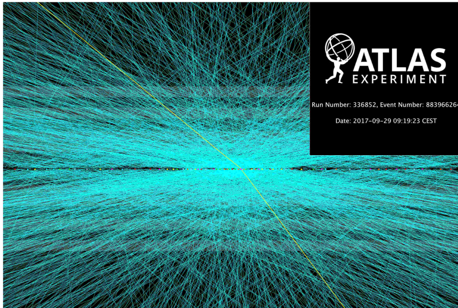
Figure 2.13. Display of the Inner Detector in a pp collision event, collected in September 2017, with a Z \rightarrow \mu\mu candidate and 65 additional vertices. Image taken from [47].
