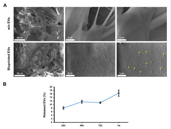
**Figure 4.** SEM analysis and *in vitro* EV release kinetic assay. (A) SEM images of 3D bioprinted hydrogels (GelMA without EVs and GelMA with EVs). Yellow arrows show a few vesicles. (B) Bioprinted EV dispersion profile in 1 week of culture in EV-free medium.
