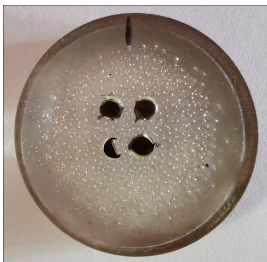
Figure 2.4. Picture of samples mounted in epoxy and polished for analysis
