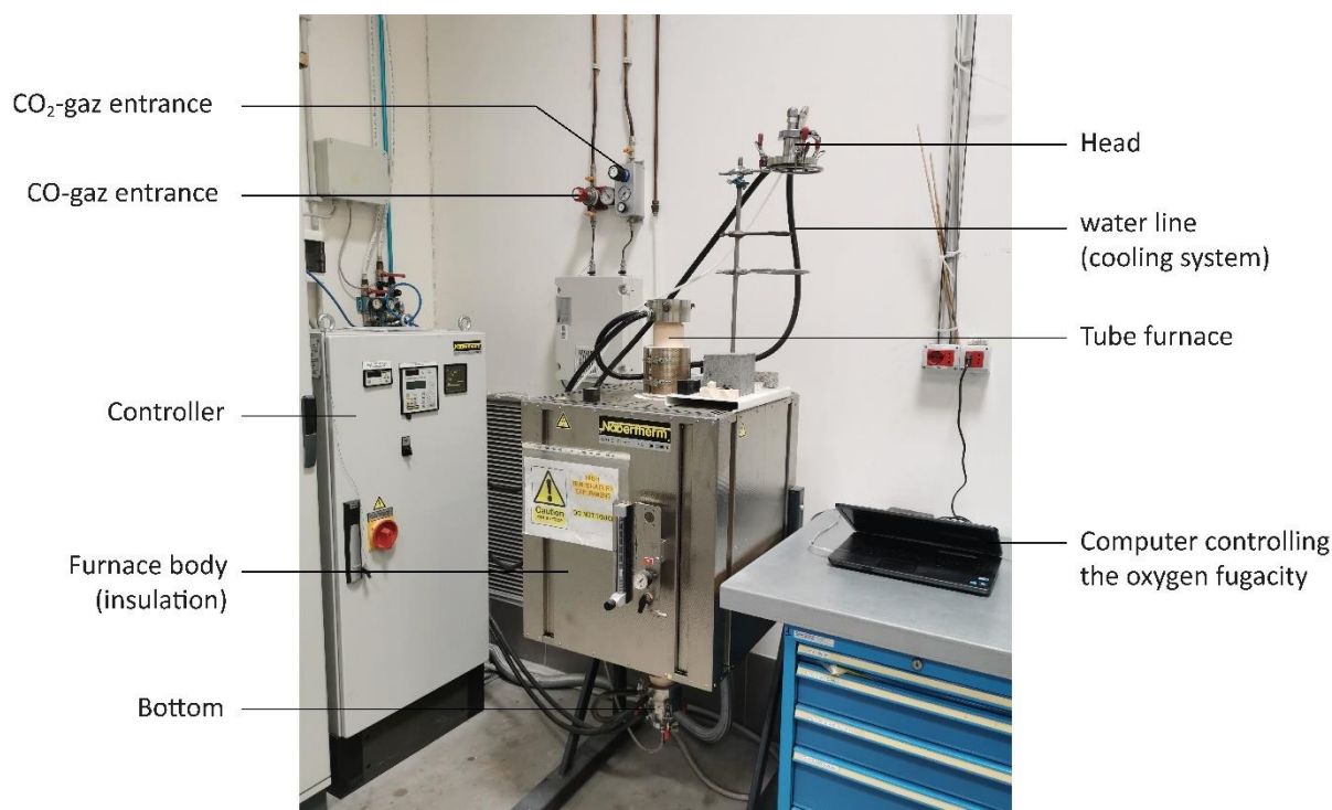
Figure 2.2. Photo of the 1 atm vertical tube CO-CO 2 gas-mixing furnace Nabertherm Furnace RHTV 120-300/18 installed at the laboratory HP-HT of INGV in Rome, Italy.
