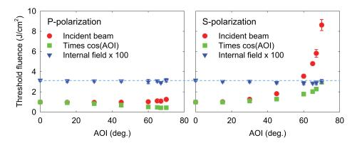
FIG. 3. Ablation threshold fluence and the quantities related to it, vs. AOI for gold. The internal fluence shown is multiplied by 100, to make it visible on the plots. The experimental errors are due to the extrapolation uncertainty at large values of the AOI.
