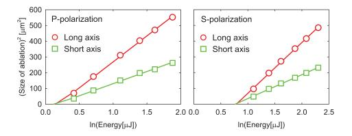
FIG. 2. Examples of the data for the size of the ablation crater squared vs. logarithm of the energy of the ablating laser pulse, for the case of a gold sample illuminated at  $45^{\circ}$  AOI. The left and right panels show P- and S-polarizations of the incident laser beam, respectively. The two lines of data on each plot correspond to the long and short axes of the elliptical ablation crater. The experimental errors in these data are small compared to the size of the data symbols.
